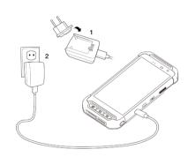
1. Insert USB connector into the adapter and connect to an electrical socket to charge.
