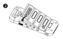
2. Insert the battery cover from the bottom first.
